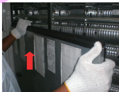
Fig 2. Remove inner door To remove inner door, lift inner door up to hinge dislodge (inner door)
